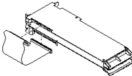
**NOTE** The connector of the vertex data bus cable can be installed in only one orientation.
